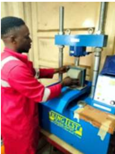
Determination of Unconfined compressive strength and indirect tensile strength on stabilized material
