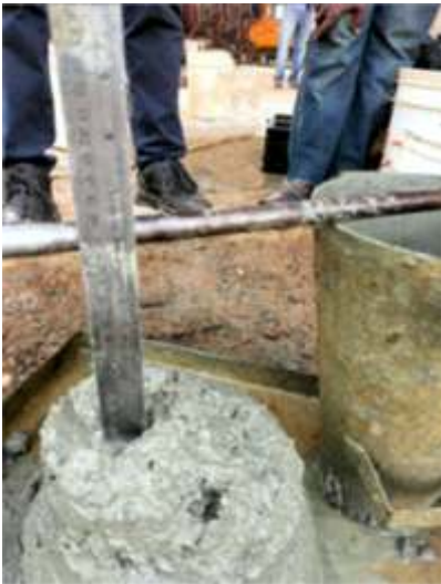
Slump test to check for the workability of the concrete
