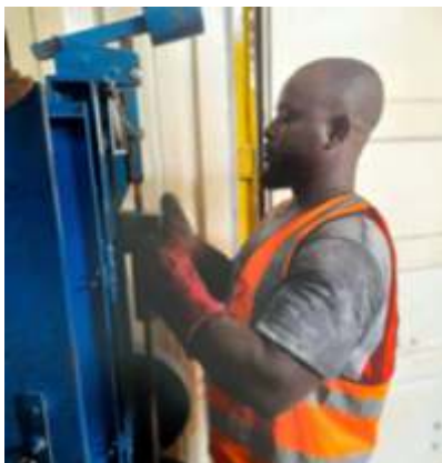
Marshall Compaction of asphalt
