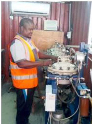
Permeability test for measuring the quantity of water percolating through the concrete Cubes during a given interval of time and computing the coefficient of permeability
