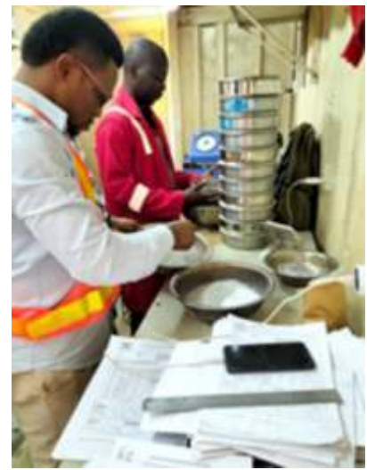
(Indicator section) Sieve analysis to assess the particle distribution of soil material allowing the material to pass through a series of sieves of progressively smaller mesh size and weighing the amount that is stopped by each sieve as a fraction of the whole material
