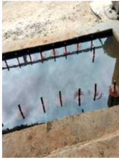
Compacted CBR specimen soaked in the water bath. The California bearing ratio test is performed in order to evaluate the strength of soil subgrades and base course materials
