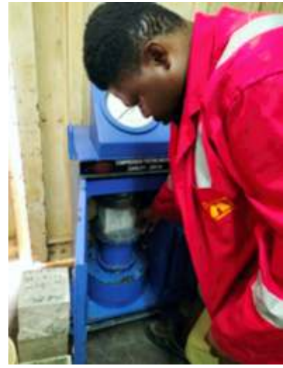
Crushing of the crushing cubes to determine the compressive strength of the concrete
