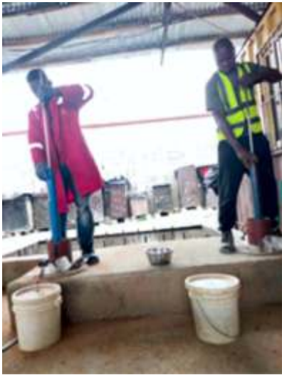
Compaction of soil materials to determine the maximum dry density and optimum moisture content of the material
