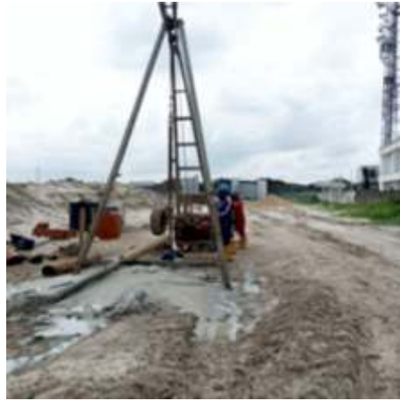
Hitech Geotechnical team carrying out soil investigation with the Dando III Percussion drilling rig. Location: REGIONAL ROAD PROJECT VGC LAGOS
